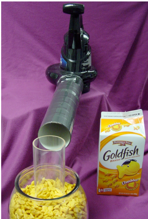
Placement of the leaf blower at a 90° angle, half above and half below the tube is crucial.
